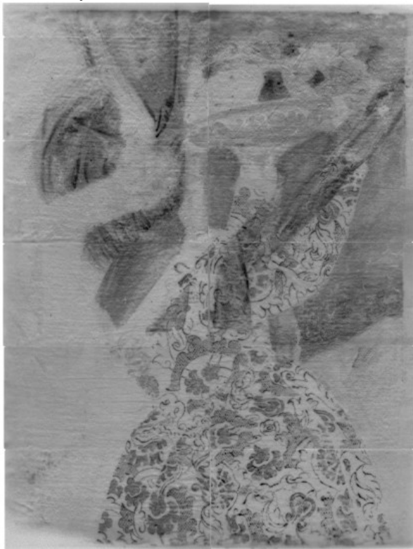
Fig. 3: 2 nd neutron autoradiography, composed of 12 imaging plates, exposure 1d 7 h to 1d 11 h after activation.
